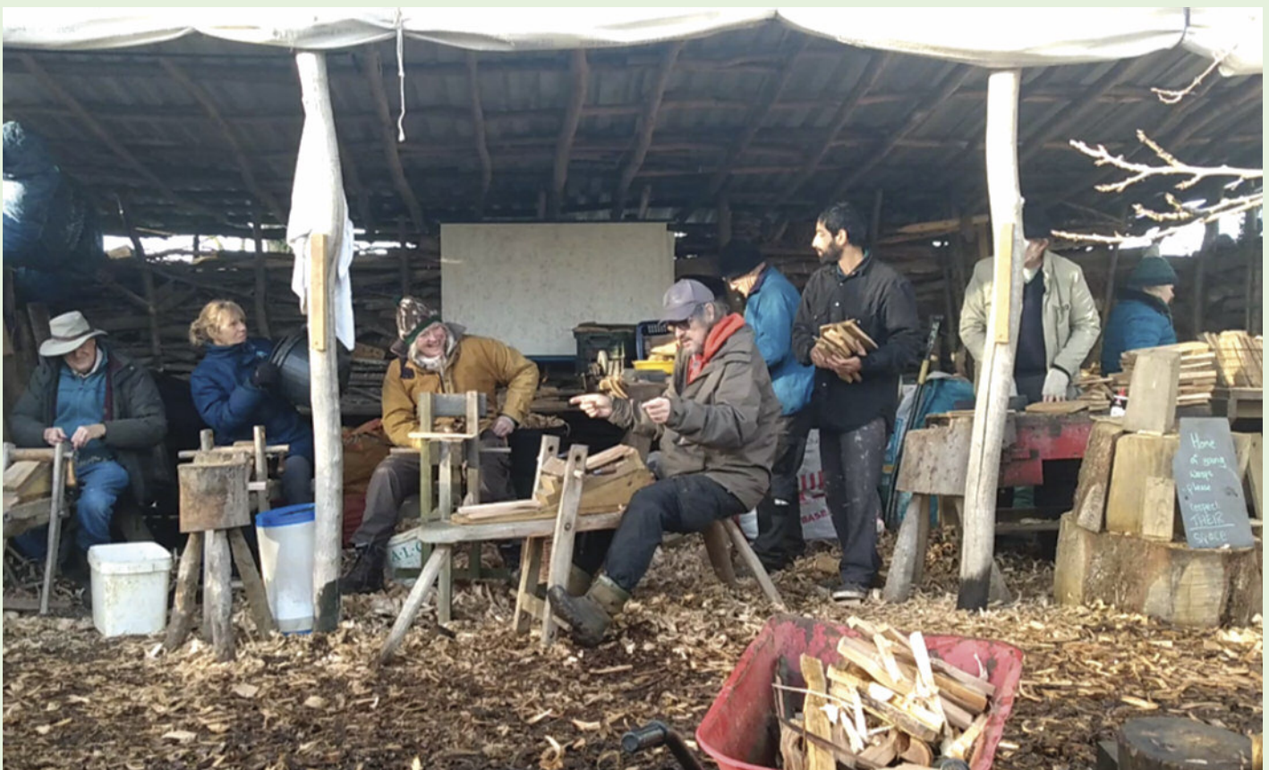
Work and play: The volunteers have fun while they produce roofing shingles
