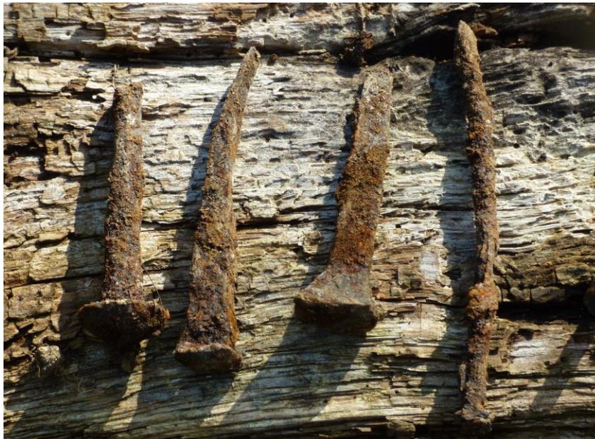
Nails as fixings were used in ancient Egypt and in the UK by the Romans and during the bronze age. During the Tudor period Iron nails were hand wrought and hammered into a square shape. In about 1600 a machine was created to automate the production. Round wire nails were produced from about 1890. Many examples have been found in the remains of the 1580 Longhouse.
